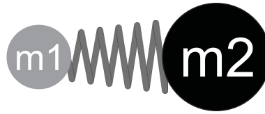
Figure 2.5: The molecular bond between two atoms m1 and m2 can be represented as a spring.
