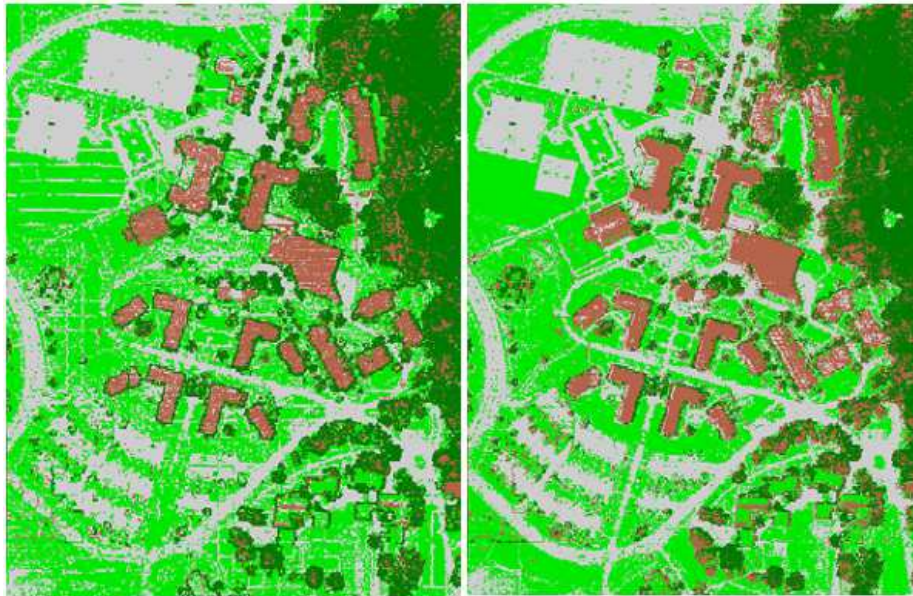
Figure 14. Classification results using LiDAR features and luminance from aerial image, left: only LiDAR features, P(\text{correct})=0.74 , right: All features, P(\text{correct})=0.85 . From [9].
