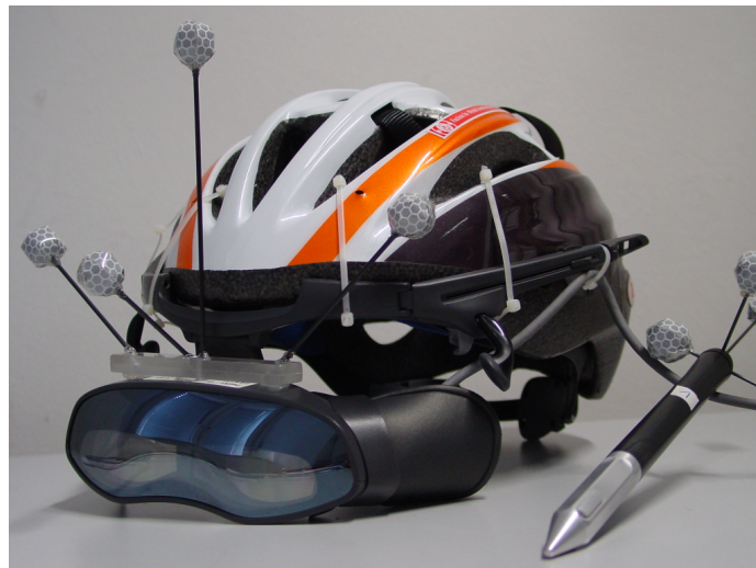
Figure 3.11: A head mounted display and pen, as typically used in Construct3D setup
