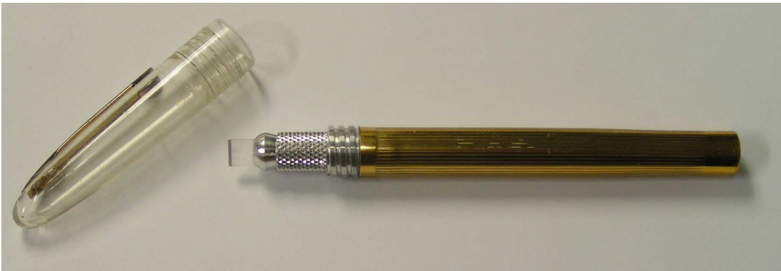
Figure 2.7.: “Sapphire Proscribe” used for wounding the coating and cladding to cleave the PBG fiber.
