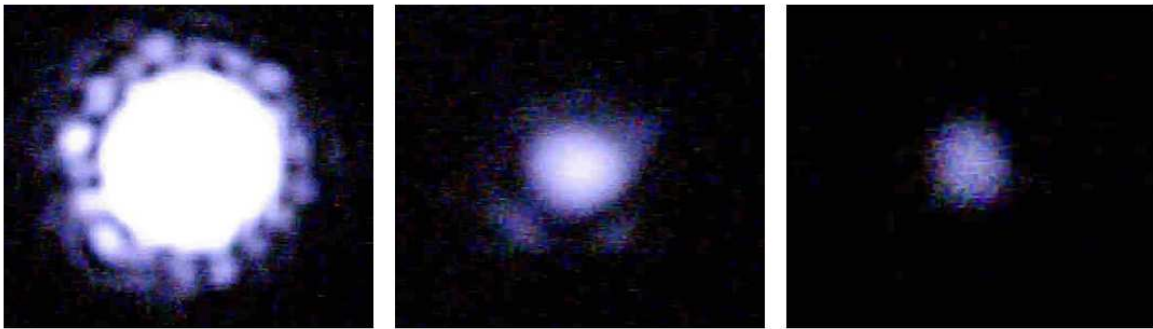
Figure 2.12.: Gradually attenuated fundamental mode at the output of the fiber. The fundamental mode is characterized by only one intensity peak.
