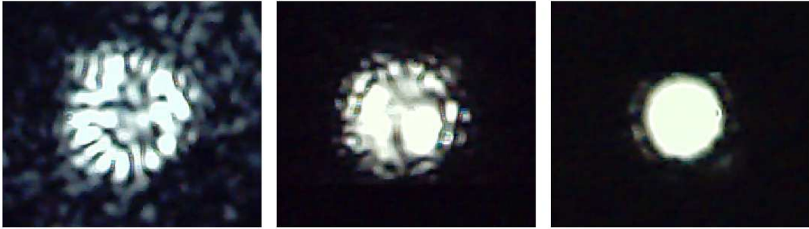
Figure 2.14.: Left picture shows the output of the fiber for a misaligned beam. The middle picture presents a bad coupling procedure, in which the screws of all directions were moved and no fundamental mode was assured. The right picture displays fully coupled beam into the hollow core of the fiber.
