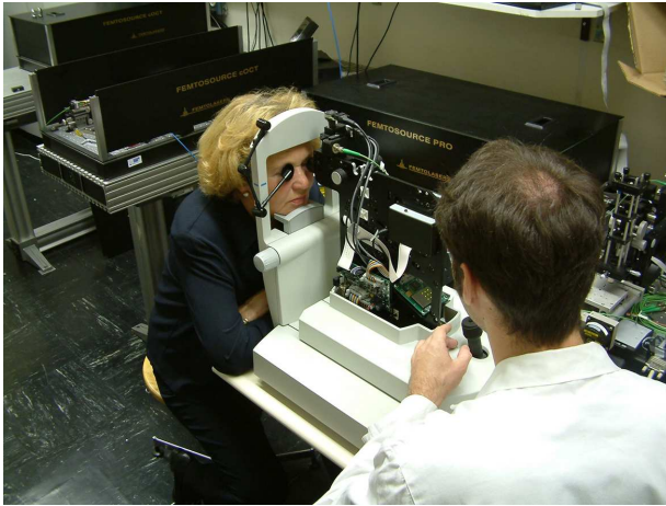
Figure 3.21: Prototype of the clinical UHR OCT system. A ultrabroad bandwidth titanium:sapphire laser (up to 170 nm bandwidth full width half maximum, 800 nm central wavelength.) is interfaced to a fundus camera (Zeiss OCT 1, Zeiss Meditec, Dublin, CA). The fiberbased interferometer and the optics of the fundus camera were designed to support the whole bandwidth of the laser.
