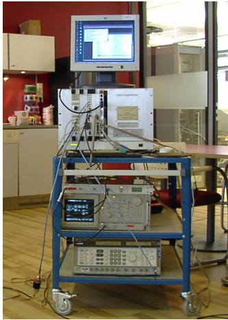
Figure 3.17: The Sintef transmitter acting as an indoor base station.
