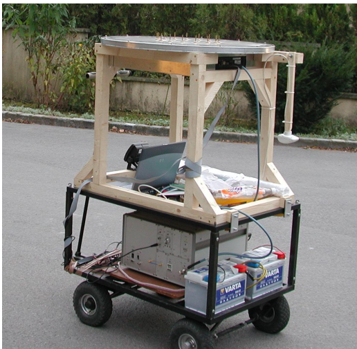
Figure 3.4: The RUSK-ATM transmitter mounted on a trolley.
