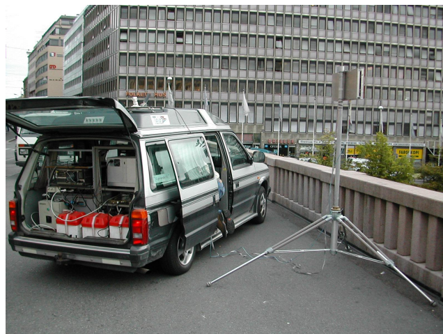
Figure 3.19: The transmitter of the Sintef channel sounder mounted inside a car. The photo shows the measurement setup for an urban microcell.
