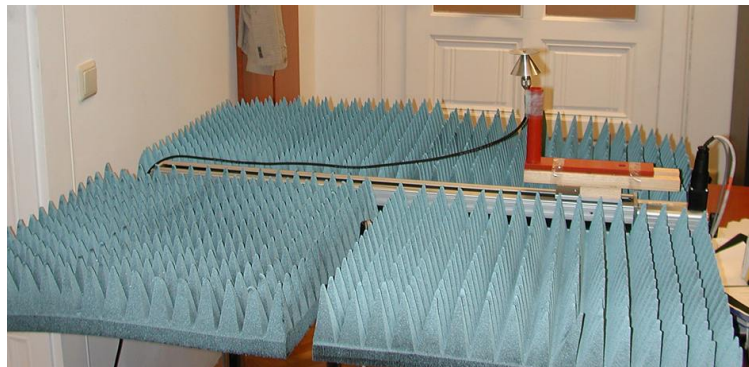
Figure 3.6: The positioning table with one omni-directional antenna on top.
