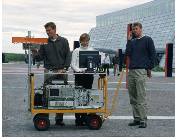
Figure 3.18: The Sintef receiver mounted on a trolley for outdoor measurements.
