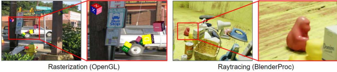
Figure 3.5: Training Data Rendering Comparison of rendering object views on top of Microsoft COCO images [34] using rasterisation (left image pair) and rendering from cluttered virtual scenes using raytracing with BlenderProc [68] (right image pair).
