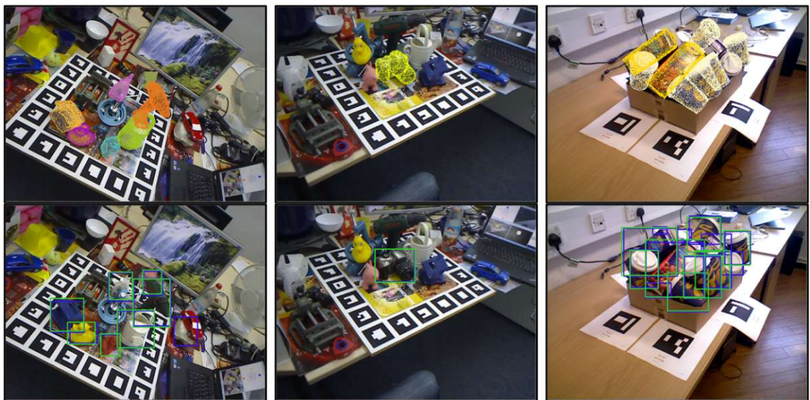
Figure 4.13: Qualitative results on Occlusion, Linemod and IC-bin. Top row shows projected object meshes based on the estimated poses, bottom row shows bounding box estimates. Blue boxes indicate the ground truth while green boxes indicate estimates.
