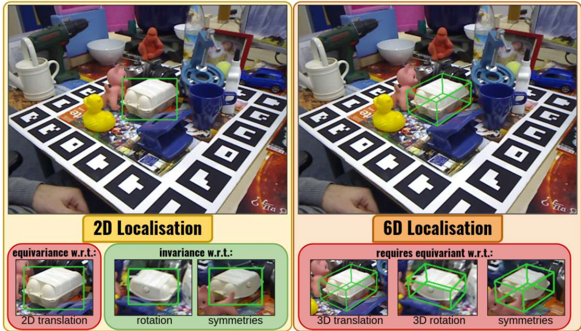
Figure 1.2: 2D versus 6D Object Localisation: Object detection, respectively 2D localisation aims to recover the rough image location containing an object of interest. This requires the learned encoding to be equivariant with respect to image space translation and scale, allowing invariant mappings w.r.t object rotation and ambiguities resulting from object symmetries. Object pose estimation, respectively 6D localisation, requires learning an encoding equivariant w.r.t. 3D translation and rotation and object symmetries.
