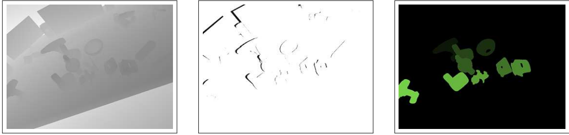
Figure 3.2: Renderer Output Synthetic depth image (left), visibility mask (middle) and pixel level class correspondence (right).
