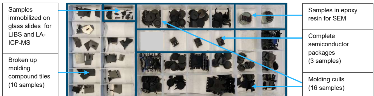
Figure 13: Depiction of all molding compound samples investigated.
