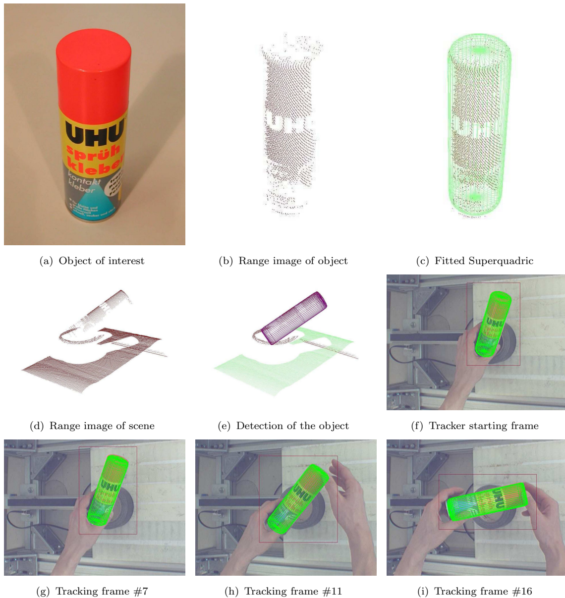
Figure 6.4: Experiment 2: Handling of a cylinder. Capturing model (first row), Detecting (second row) and Tracking (last row). The reprojected pose is depicted as mesh-grid.
