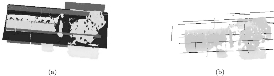
Figure 3.4: (a) Generation of the main faces on the motor and gearbox (reduced VRML format). (b) Calculated paint strokes located on the main faces.
