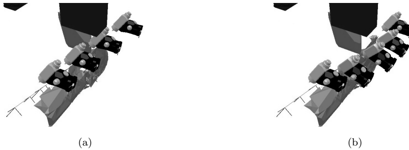
Figure 3.5: (a) Original paint trajectory generated by the PaintPlanner. (b) Paint trajectory after it has been modified by the ToolPlanner.
