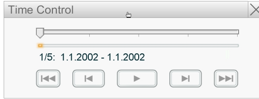
Figure 4.17: The time control window in Gravi++ lets the user select a specific timestep, move through time, and gives feedback on the current position in time.
