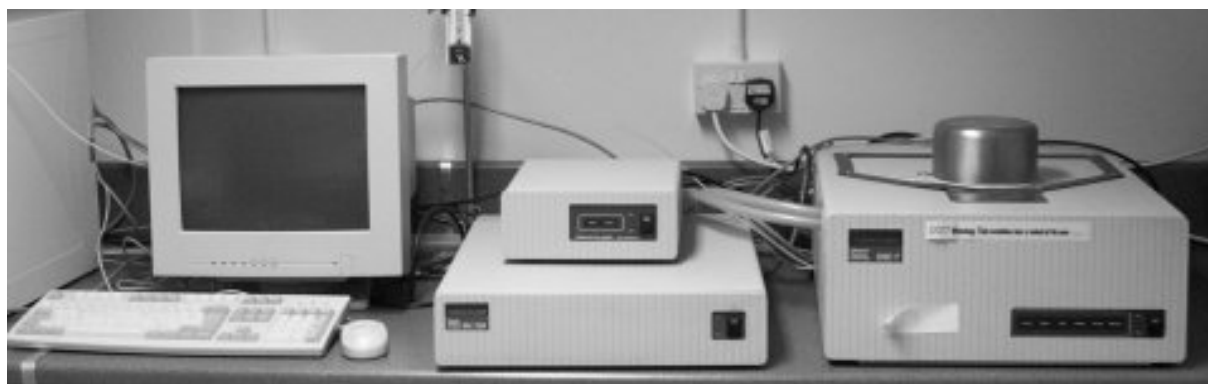
Figure 4.8. General view of Perkin-Elmer DSC7 device.
