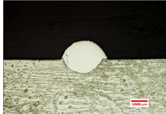
Figure 64: Deeper weld bead penetration in case LB
