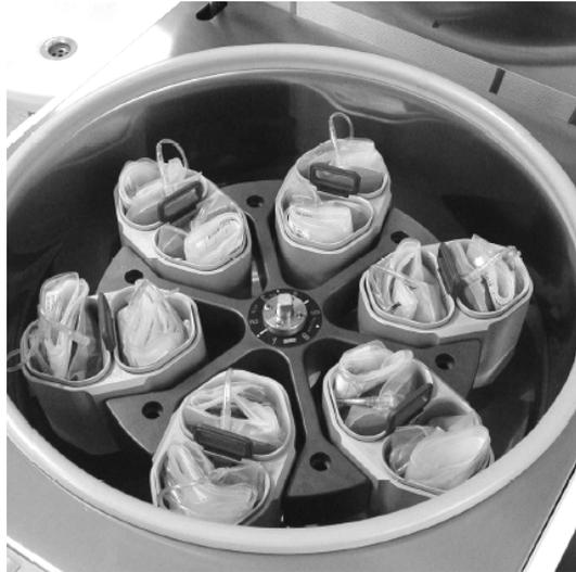
Fig. 28: Blood bag systems in the centrifuge [Wagn06a]
