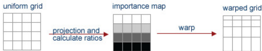
Figure 3.19: The basic steps involved in the grid warping algorithm. Image courtesy of [34].
