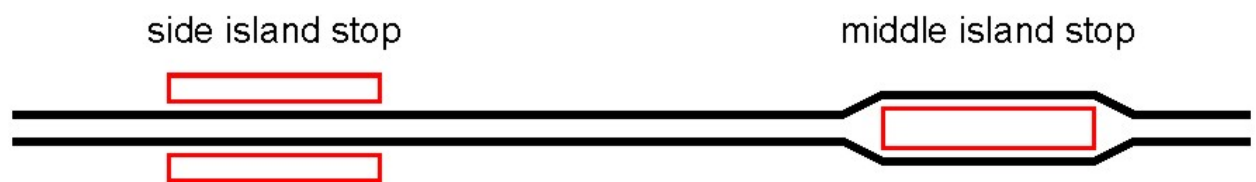
App.fig. 10: Stop island types. According to (Etzold 1999a)
