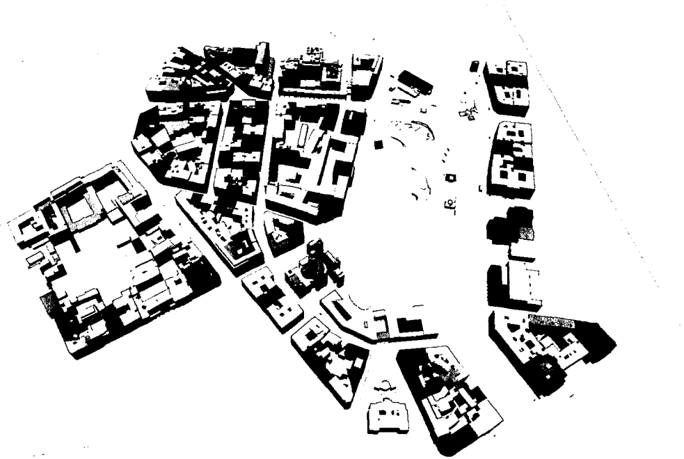
Figure 8.10: A subset of the 3D model of the City of Vienna. It includes a digital elevation model, building blocks and roofs. 3D model courtesy of Vienna City Administration.
