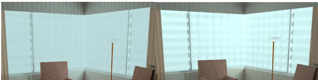
Figure 8.6: Particular of the window in the Hotel room image: (left) without visual acuity, (right) with visual acuity. The details in the window (image on the right) are more visible and in particular the bulb of the lamp is well defined.
