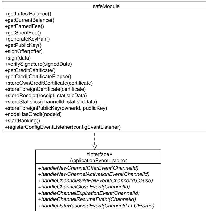
Figure 3.31: Overview over the safe module's functions
