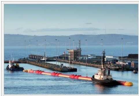
Figure 3-7 Wave energy converter 34
