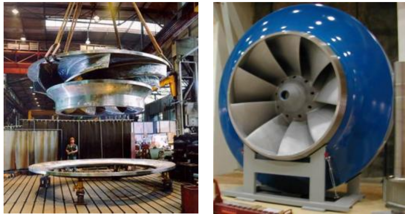
Figure 7-3 Pump-turbines of Goldisthal 133
