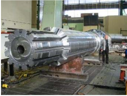
Figure 7-4 Shaft of the DFIM Goldisthal 134
