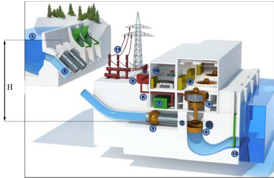
Figure 3-1 Details of a typical storage power plant 20
