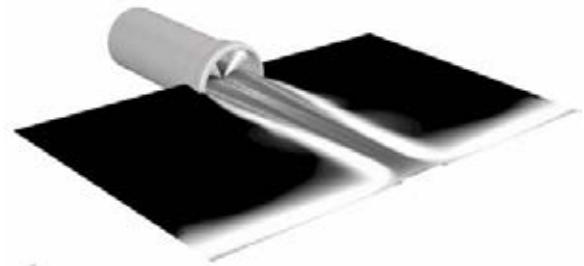
Figure 2: Turbulent kinetic energy [ m^2/s^2 ] for a turbulent generator with 4 spikes. The simulations are performed using a steady k\epsilon -RNG model (grey scale range from 0 to 1).
