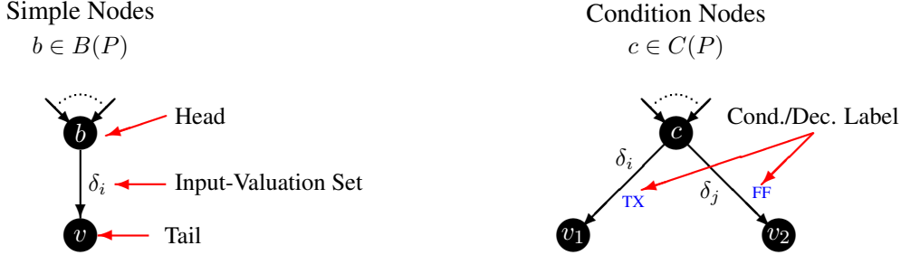
Figure 3.1: Components associated with an edge e of an aCFG representing a program P , dependent on the type of statement represented by head(e) .
