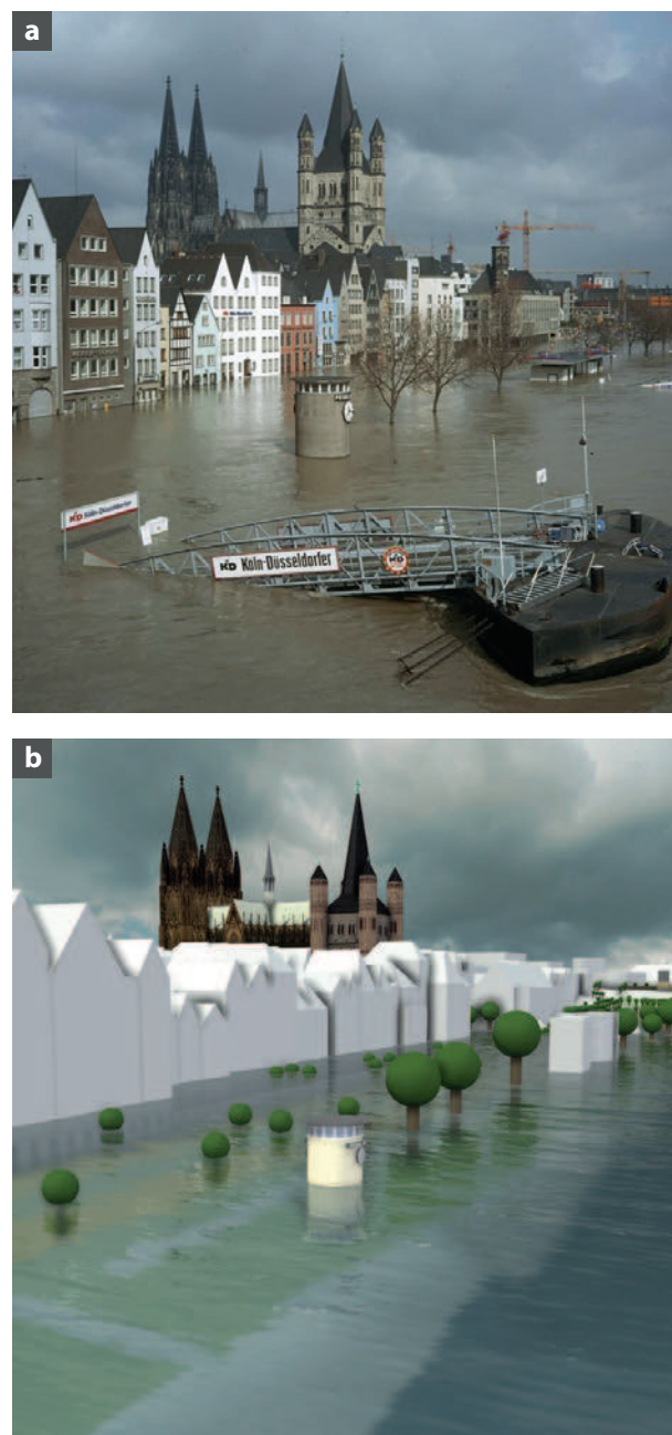
Figure 4.10: Comparison of real flooding with our technique. (a) Turbid water in reality makes it impossible to identify completely inundated structures and to estimate water depths. (b) Our technique provides a geospatial context by revealing inundated structures such as streets and floodwalls.
