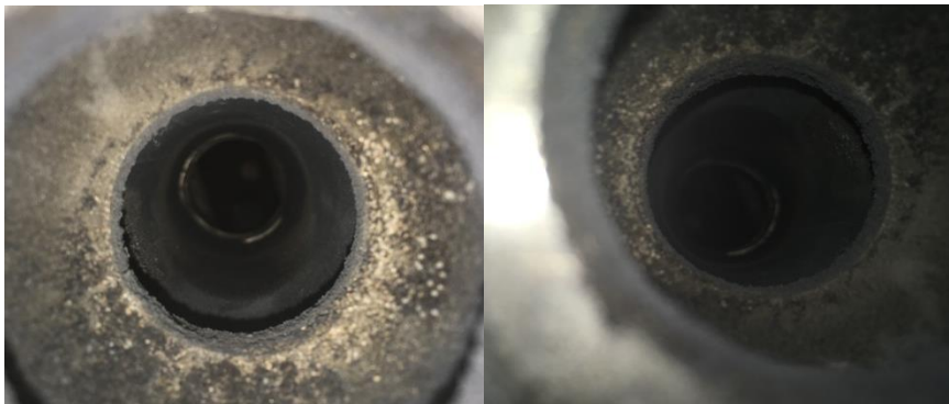
Figure 25: Bench-scale reactor after experiment with wheat straw, deposit formation
