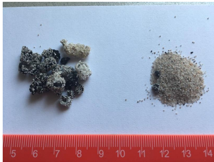
Figure 17: Wheat straw combustion - the agglomerates (left) and the bed material (right); 300 g of bed material
