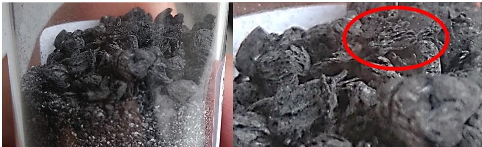
Figure 29: Ash residues from the experiment with non-pelletized lignin
