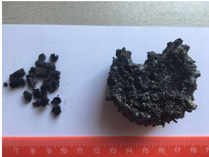
Figure 18: Wheat straw combustion - single large agglomerate; 50 g of bed material
