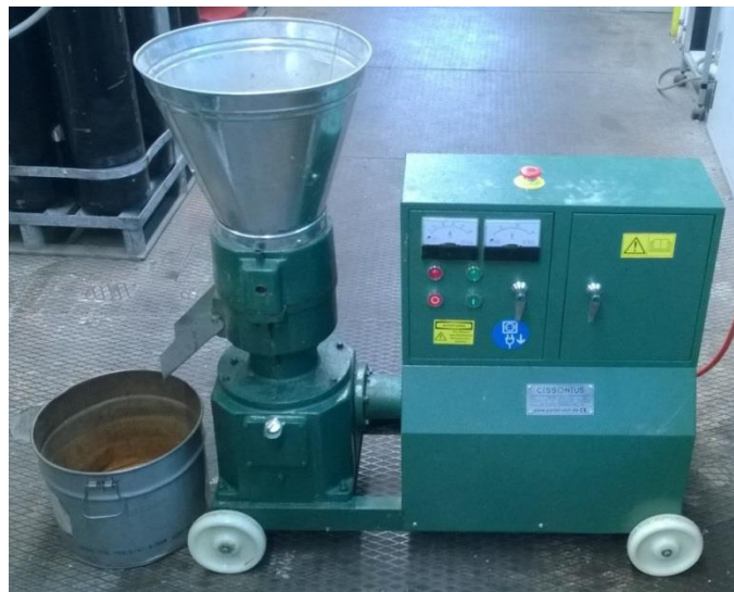
Figure 9: Pelletizer from company Cissonius with electrical power of 7.5kW
