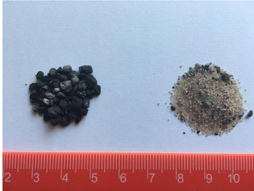
Figure 21: Combustion of lignin in the lab-scale reactor - Sample of the ash (left) and the bed material (right)
