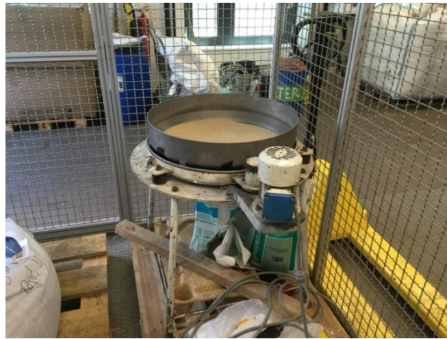
Figure 11: Vibration sieve from Fuchs Mühlen
