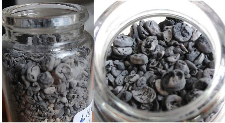
Figure 28: Ash residues from the experiment with pelletized lignin
