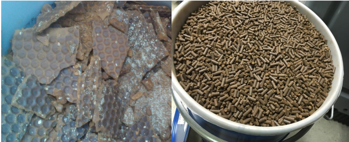
Figure 10: Wheat straw lignin before and after pelletizing
