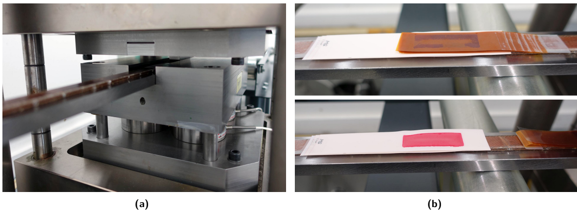
Figure 3.4: (a) Picture of specimen 1 (cable HT15OC0190) in the pressing tool and (b) 1 mm thick Polyimide foil stack intermediate layer (top) with pressure-sensitive films (bottom) after applying a nominal stress of 175 MPa.
