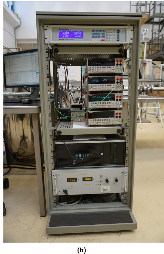
Figure 3.17: Measurement and control system. (a) Schematics and wiring of equipment. (b) Picture of measurement tower installed next to the cryostat.
