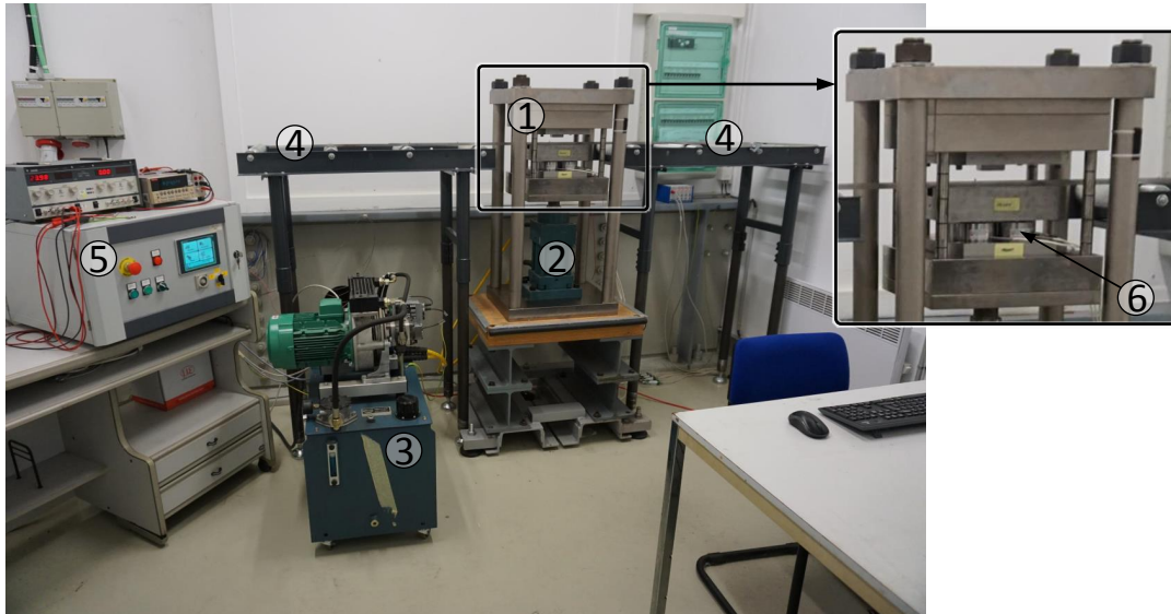
Figure 3.1: Picture of the setup for applying transverse compressive stress on the cable and wire specimens. 1. Pressing insert, 2. Hydraulic jack, 3. Hydraulic circuit, 4. Supports with support bar, 5. Control unit, 6. Load cells.
