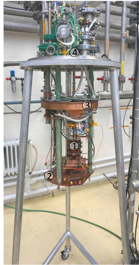
Figure 3.13: (a) Schematic of cryostat setup assembled in a vacuum chamber including sample holder and cryogenic peripheral (b) Picture of the cryostat setup outside the vacuum chamber. 1. Phase separator, 2. Experiment platform, 3. Fixation for thermal shield, 4. Electrical and cryogenics feed-troughs.
