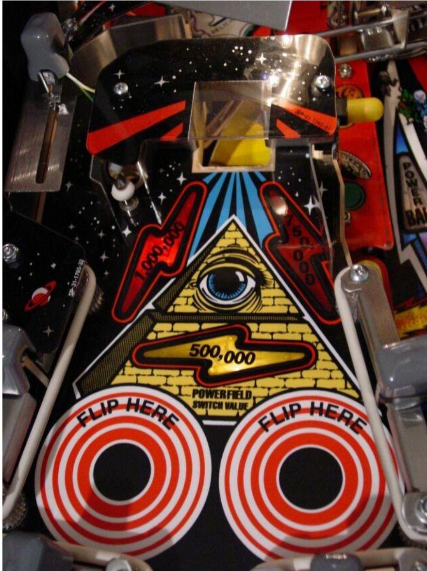
Figure 6.14: The mini-playfield of the pinball game “Twilight Zone”. It uses two electromagnets to simulate the flippers.
