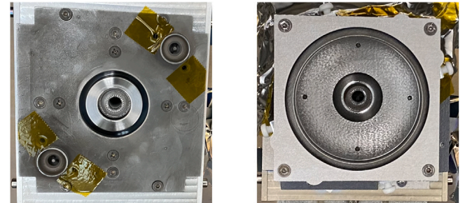
Fig. 8. Close-up view of IFM Nano Thruster laboratory model (left) and with attached focus module (right).
