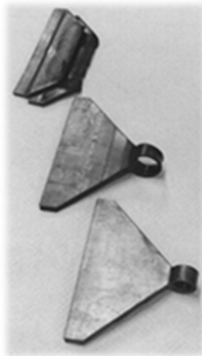
Figure 2.6: 12mm \times 12mm \times 3mm stcs before the experiment (bottom), after a 10 kV, 6 kJ discharge with 37 T peak field (middle) and after a 55 kV, 189 kJ discharge with 188 T peak field (top).
