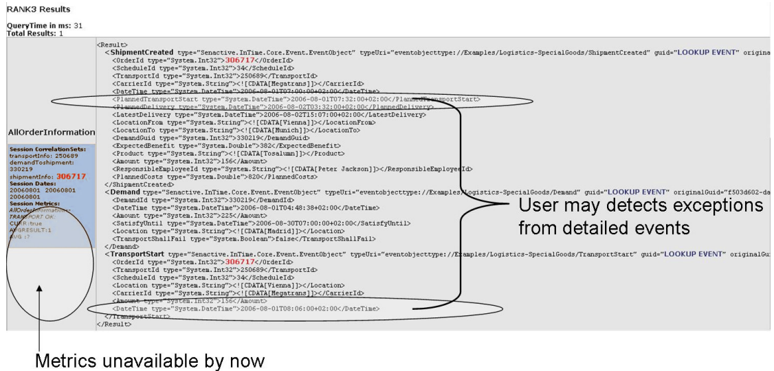
Figure 8.5: Current status of Shipment 306717. The shipment’s correlation instance is available immediately in EventCloud
