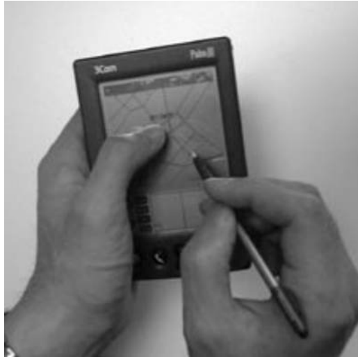
Figure 7: Two-contact handheld interaction with DualTouch [75]
