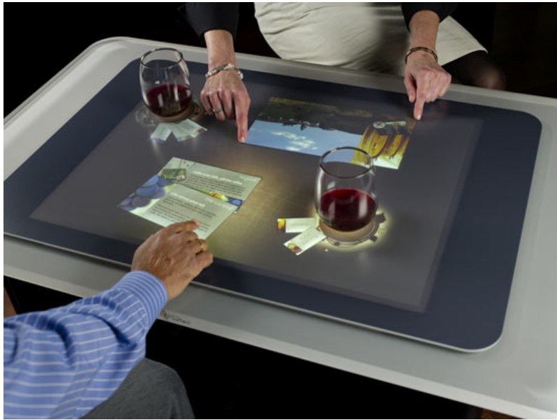
Figure 10: Near-infrared vision-based touch sensing with Microsoft Surface [19]
