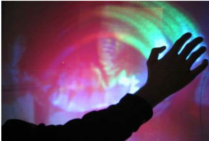
Figure 15: Touch tracking with stereo cameras on TouchLight [123]
