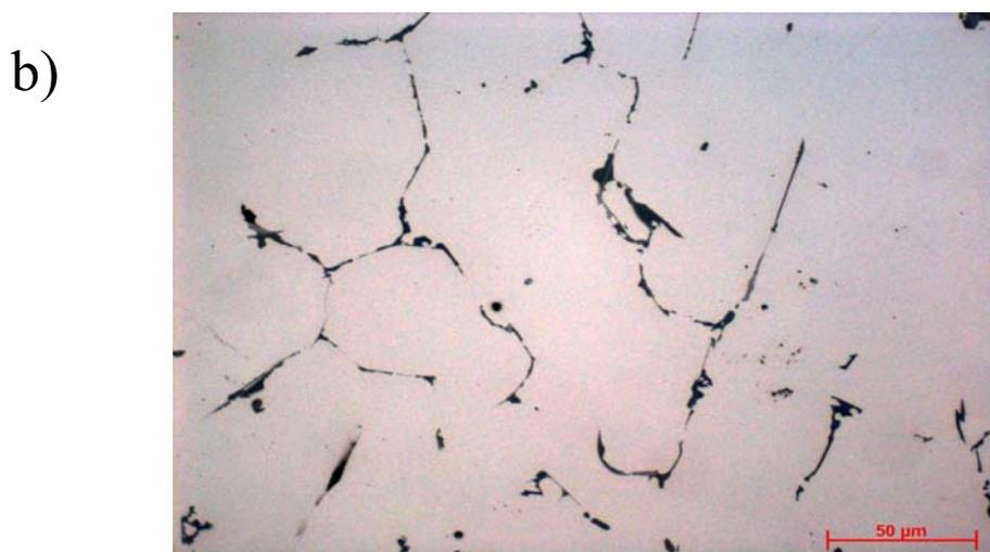
Figure 5.3 b) Light optical micrograph of Al Si1Ge5 with low Si content in as cast condition.
