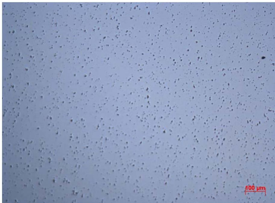
**Figure 5.20** Light optical micrograph of a cross section of extruded AW6008 with particles evenly distributed in the matrix.
