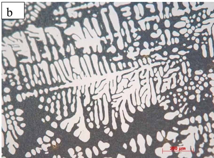
Figure 5.12 Microstructure of a) AlSi1.7 showing little interdendritic eutectic b) AlSi12 as cast condition ( $\alpha$ -Al white, eutectic Al-Si structure, dark).
