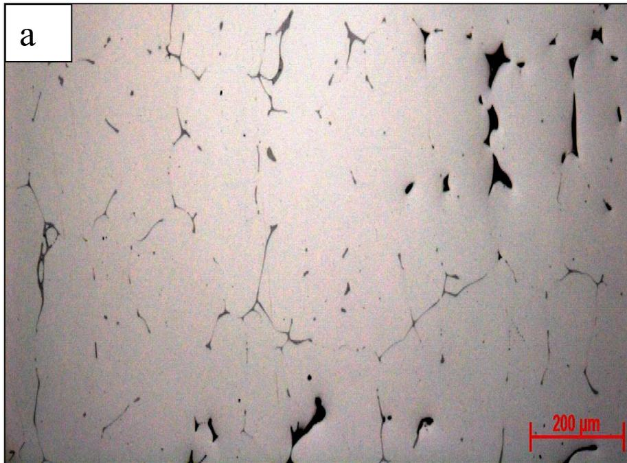
Figure 5.1.(a) Light optical micrograph of Al-Ge as cast alloy showing some porosities
