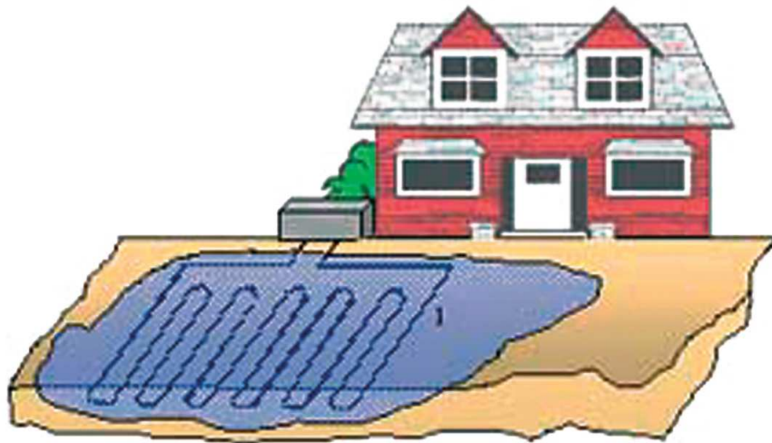
Figure no.3: Principle of the heat pump using a system of collectors
