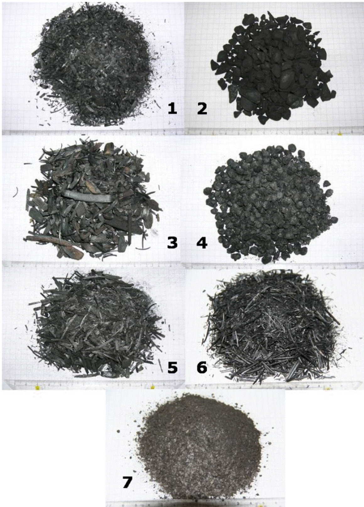
Figure 6-2: Different pyrolysis char samples from the pilot plant:(1) palm nut shells, (2) reed straw, (3) sorghum straw, (4) straw pellets, (5) miscanthus, (6) Waldviertler energy grass, (7) paper residual material
