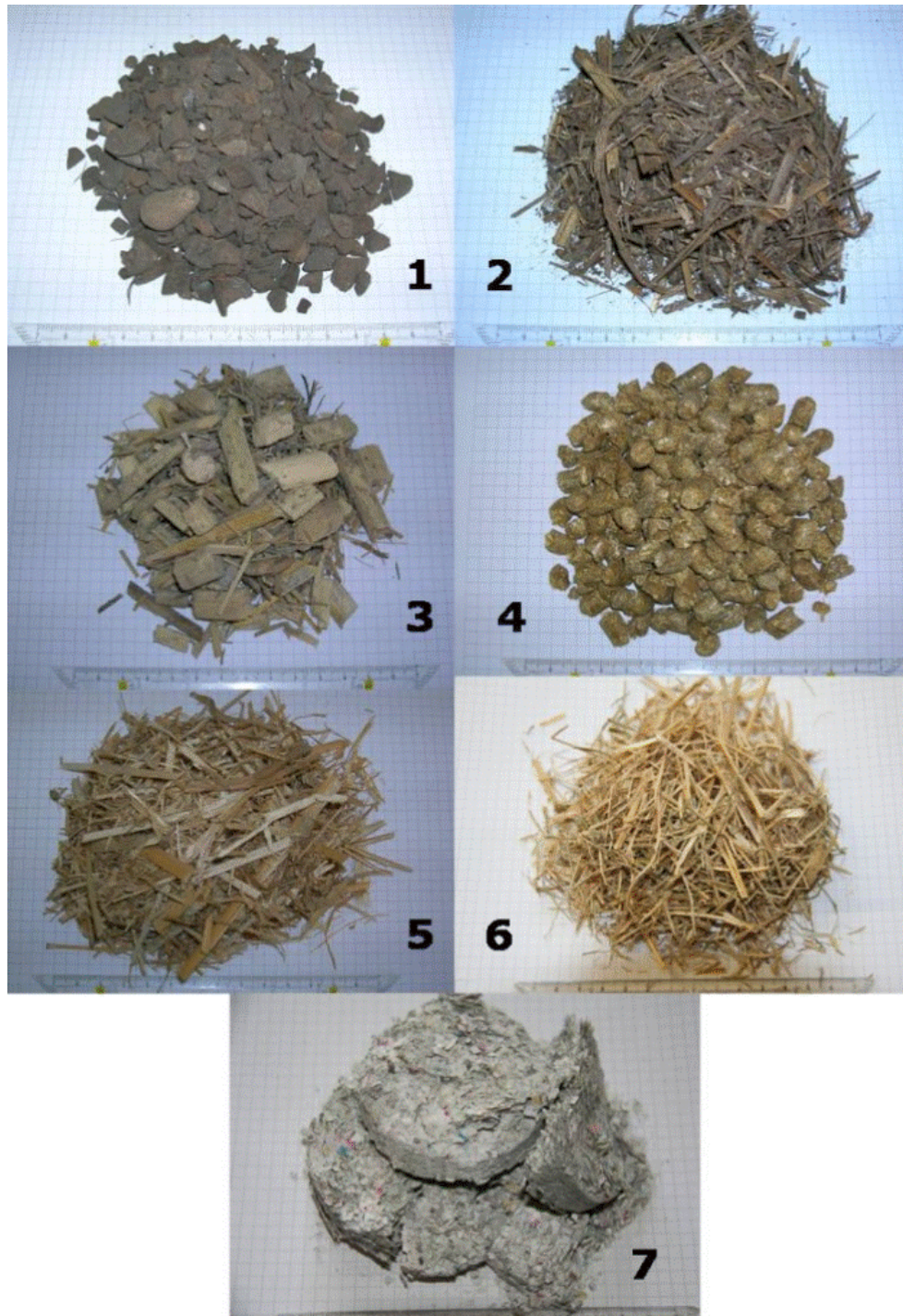
Figure 6-1: Different fuel samples:(1) palm nut shells, (2) reed straw, (3) sorghum straw, (4) straw pellets, (5) miscanthus, (6) Waldviertler energy grass, (7) paper residual material
