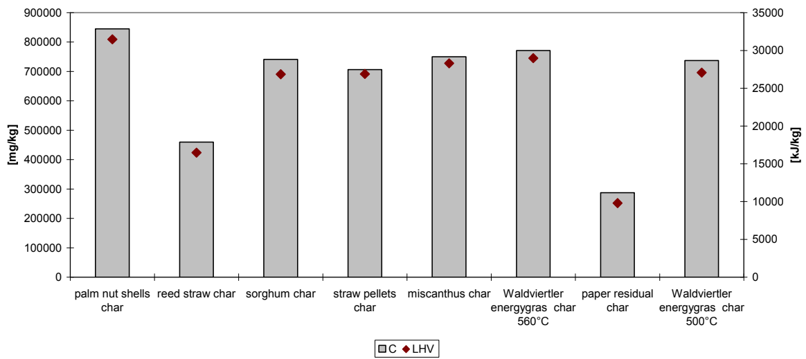
Figure 6-4: Carbon content and LHV of different pyrolysis char samples (dm)
