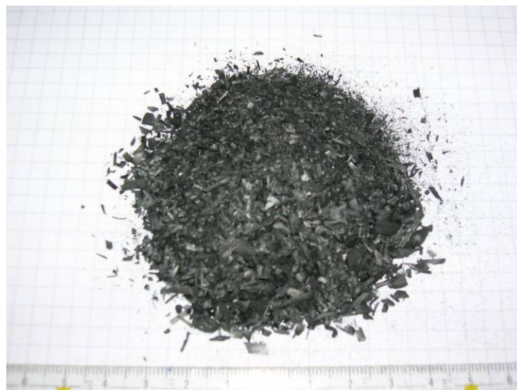
Figure 6-42: A typical pyrolysis char from the feedstock straw
