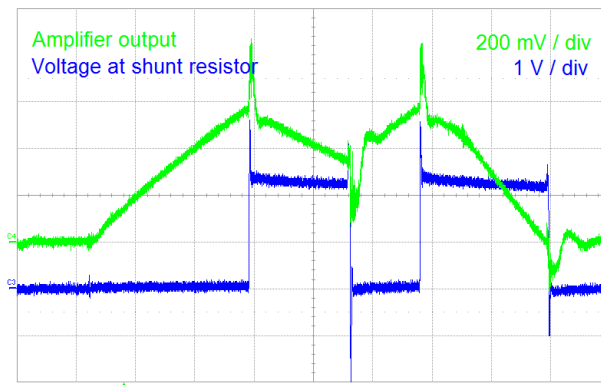
Figure 4.4: Impact of the shunt resistor's common mode voltage over- and undershoot to the current sense amplifier output
