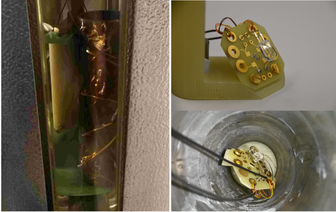
Figure 1. Experimental setup build up at the Cryogenic Laboratory at CERN. Left side: picture of the LHe bath cryostat with a viewport showing one of the Pb tubes and the adjacent magnet holder. Right side: picture of the outer Hall sensor and LED mounted on a PCB board. The SmCo magnet is seen in dark gray mounted next to the PCB. The magnetic field produced by coiled cables is below 10^{-8} mT. The lower picture shows the Hall sensor and the Chip inside the long lead tube.
