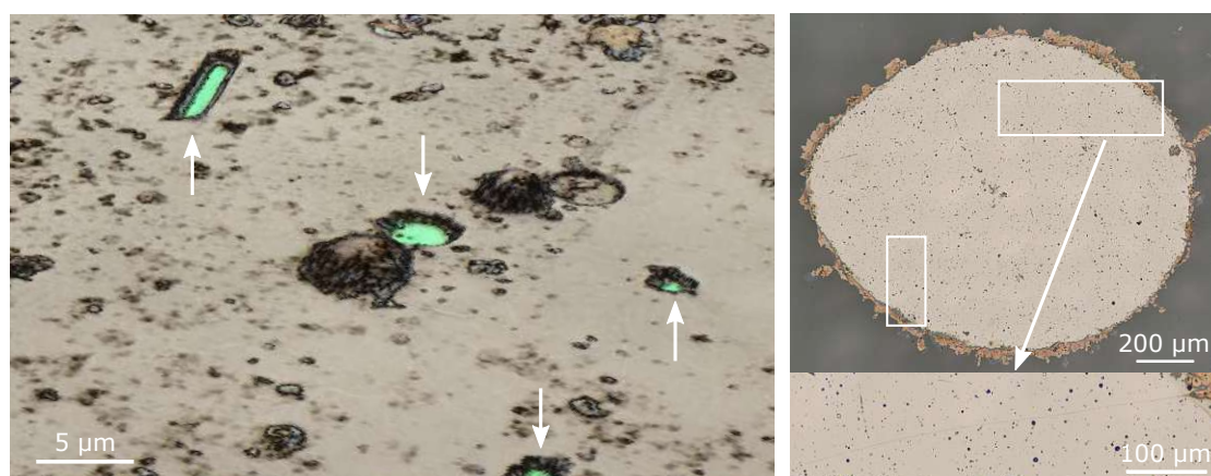
Figure 3.2.5: Digital light microscope images of the FST films on IBAD-MgO and CaF 2 . Small holes can be found in the superconducting film on IBAD-MgO, indicated by white arrows (left panel). Micro cracks can be detected in the FST film on CaF 2 (right panel).
