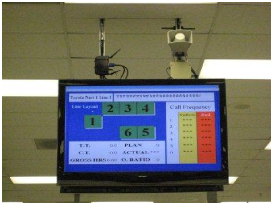
Figure 5-16: Andon board on the shop floor
