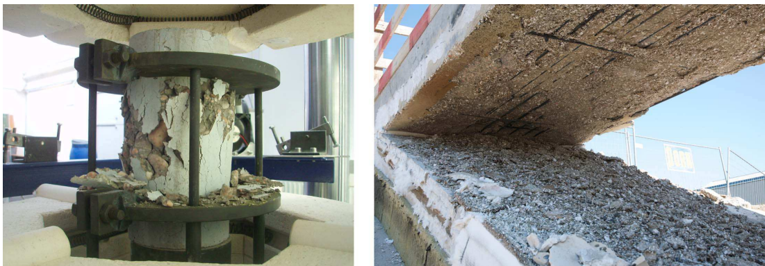
Figure 1: (a) Failure of a specimen in small-scale experiments (test of cylindrical specimens subjected to combined mechanical and thermal loading), (b) final state of spalling after large-scale fire test exposing the reinforcement bars
