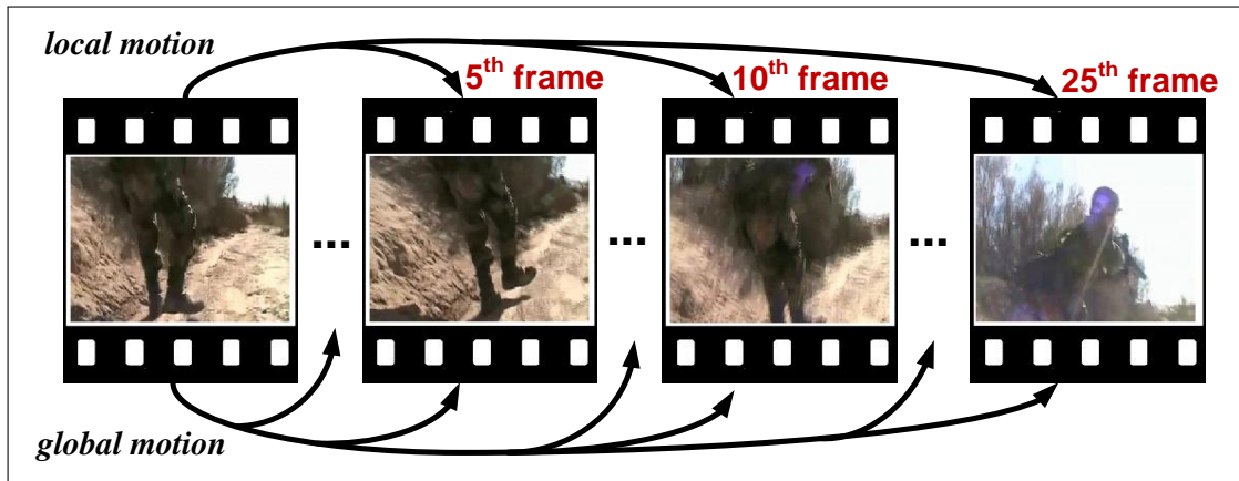
Figure 4.10: Motion features extraction. The difference of an investigated frame (leftmost one) to the frames of the following second are captured by global gist (lower arrows) and local SIFT features (upper arrows).
