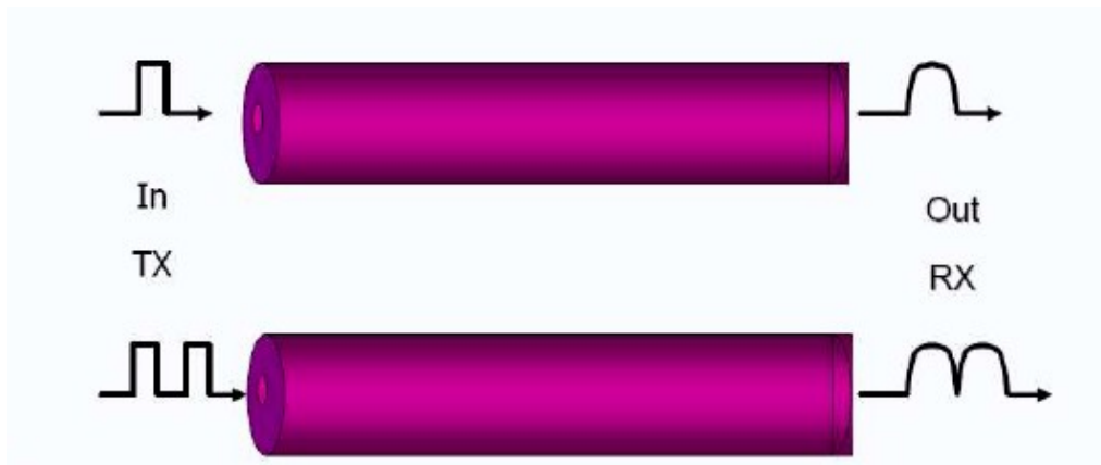
Figure 3a: Variation of the signal light pulses.
