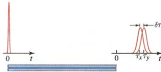
Figure 18: Differential group delay (DGD) associated with polarization mode dispersion (PMD).
