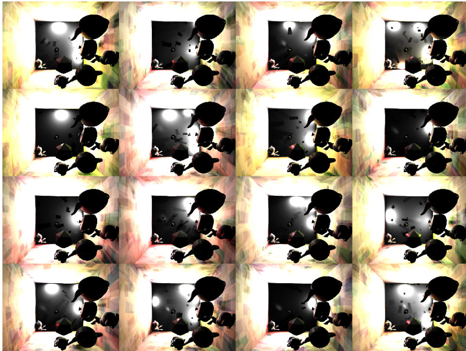
Fig. 3.4: This figure shows the accumulation buffer after shading with all VPLs. To get the final illumination the accumulation buffer must be merged, so that it does not contain any tiles anymore. Afterwards a geometry aware box filter is used to smooth indirect illumination over n \times n pixels.
