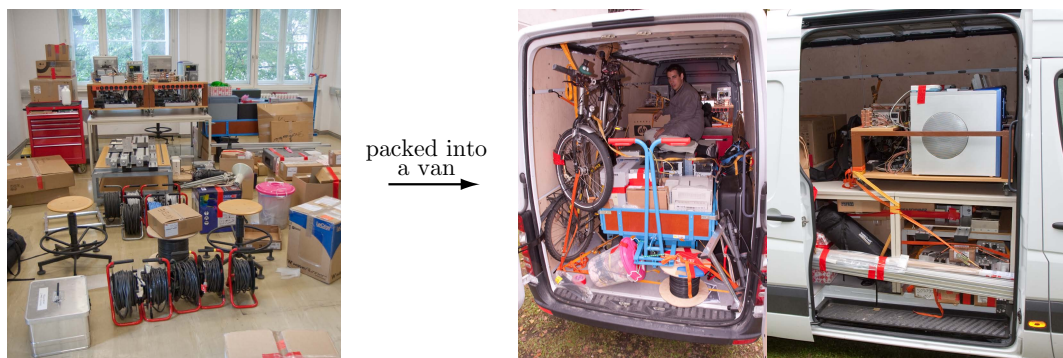
Figure 3.4: For carrying out a measurement campaign, the testbed and a small PC cluster is transported in a van.
