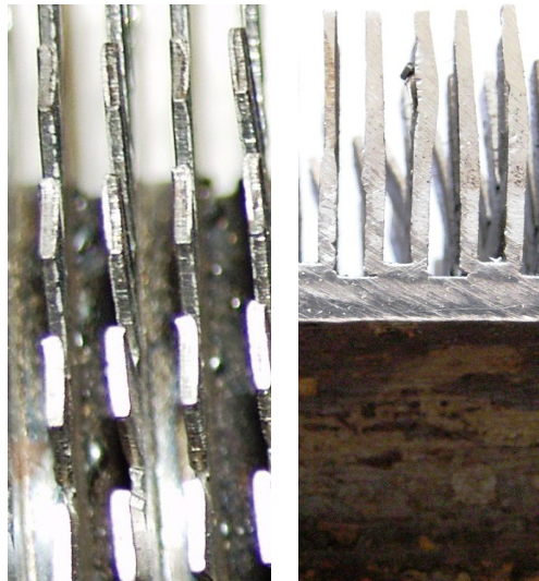
(b) Torsion of the Fins
