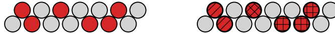
Figure 1.10: Clustering process for six individual fibers firing (marked in red). The raw fibers are shown on the left and the clusters, marked by the hatching, on the right. The leftmost cluster has the typical shape one would expect. The middle “single-fiber” cluster can occur as a result of inefficiencies in the lower layer or a dark count causing in a single fiber to fire. The rightmost cluster can be the result of a particle track crossing the fibers at a shallow angle.
