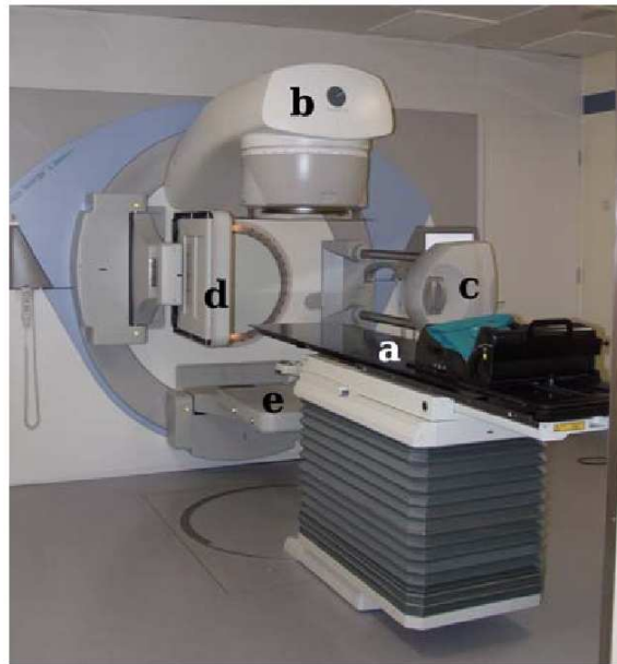
Fig. 3: An Elekta Synergy IGRT System in the Department of Radiation Therapy of the Medical University Vienna. (a) is the patient support and (b) shows the Linear Accelerator (LINAC) itself. (c) and (d) are the kV-imaging support for Image Guided Radiation Therapy and (e) is the Electronic Portal Imaging (EPI) detector for the acquisition of MV-images.
