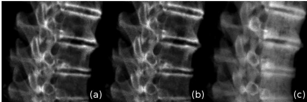
Fig. 33: Example for the z-orthogonal wobbling error of the focus wobbled splat rendering algorithm. All three images show the spine dataset rendered from a view orthogonal to the z-axis. While wobbling splat rendering using voxel wobbling (a) shows no high-energy artifacts, GPU (b) as well as CPU (c) based wobbling splat rendering with focus wobbling suffer from significant artifacts.
