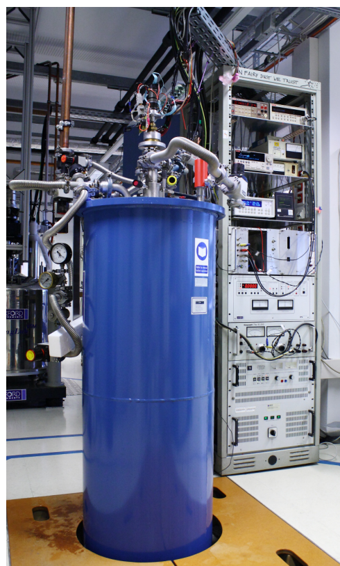
Figure 3.31.: Cryostat containing the superconducting magnet, and a rack full of equipment required to operate it.
