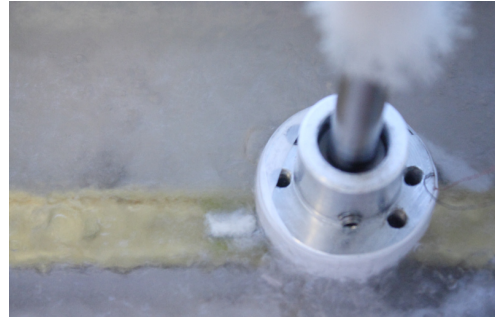
Figure 3.24.: Close-up picture of the head of the magnetoscanner during a scan.
