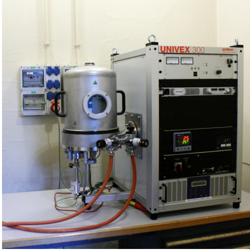
Figure 3.16.: The sputtering machine in operation. The two tubes are connected to argon and oxygen gas cylinders.
