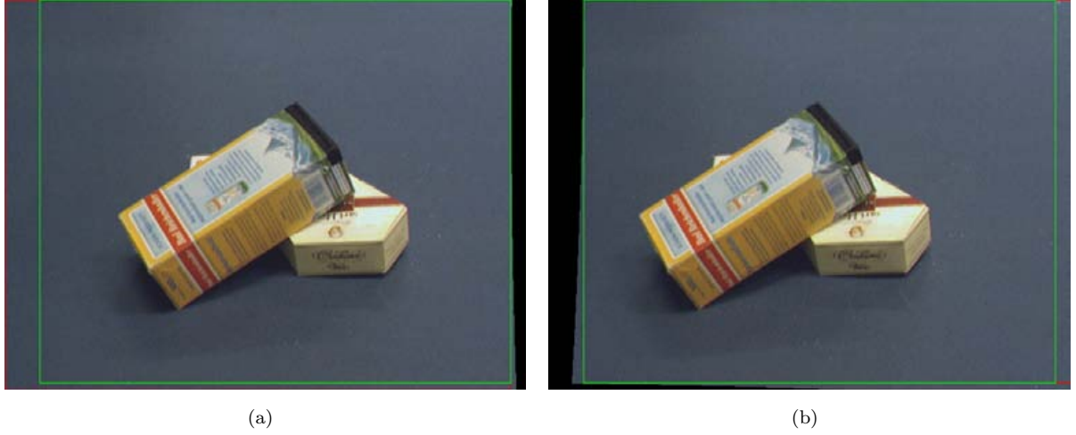
Figure 5.20: Result of the correction of the image distortion and rectification on the (a) left and (b) right image.
