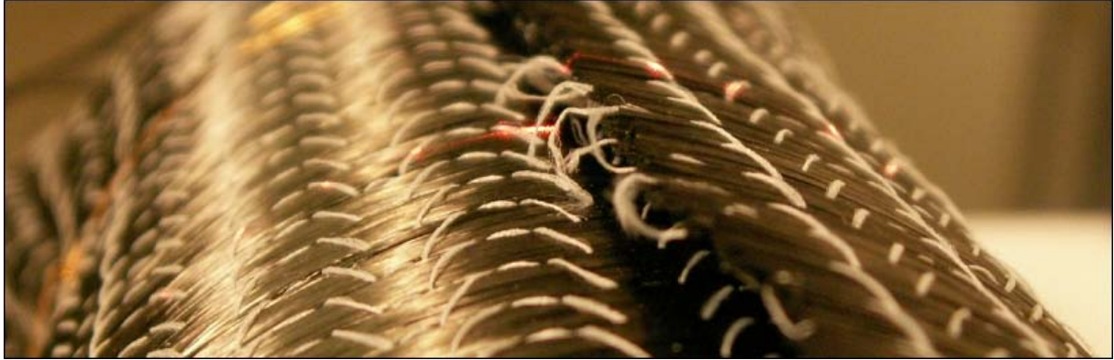
Figure 3.29: Fibre mats draped on a cylinder with a radius of 30mm.
