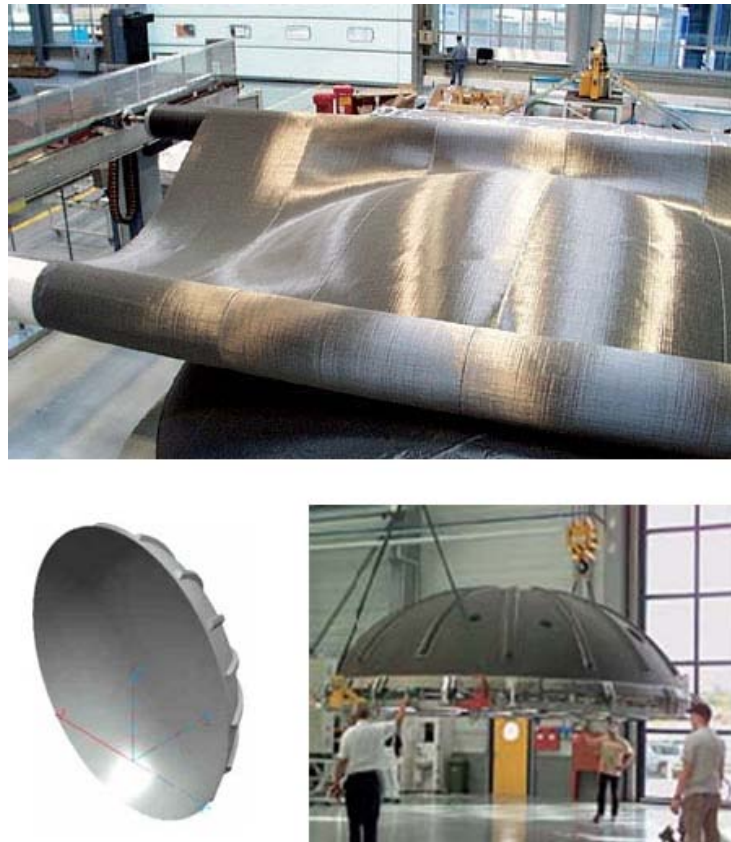
Figure 3.6: Airbus A380 rear pressure bulkhead fabricated with CFRP composites.
