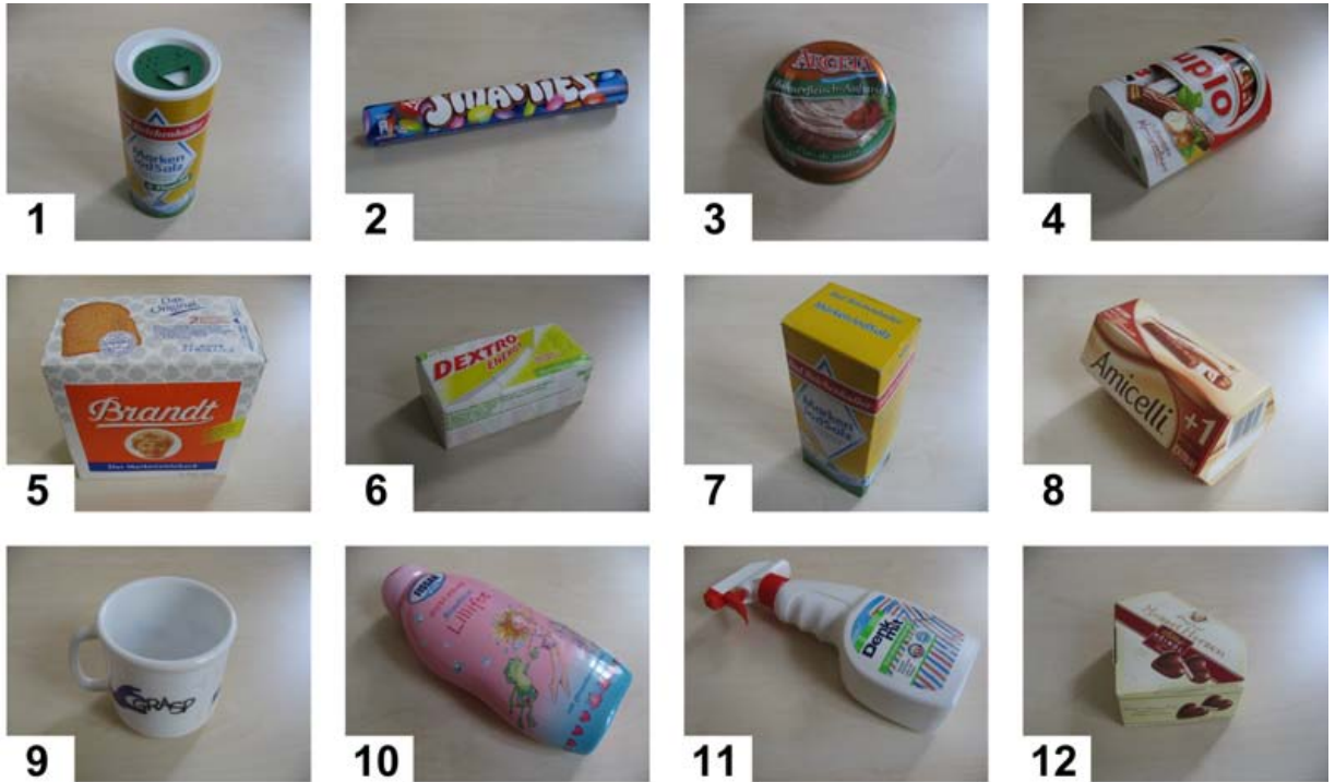
Figure 5.16: 12 different objects were selected to evaluate the grasping point and pose detection algorithm, from left: 1. Salt Shaker (cylinder), 2. Sweets (cylinder), 3. Spread (cylinder), 4. Sweets (half cylinder), 5. Melba Toast (cuboid), 6. Dextrose (cuboid), 7. Salt Shaker (cuboid), 8. Sweets (pentagon object), 9. Coffee Cup, 10. Shower Bath Gel (paraboloid), 11. Cleaner (paraboloid), 12. Sweets (prism).
