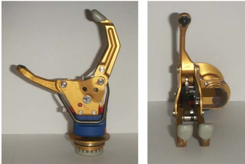
Figure 4.2: Hand prosthesis of the company Otto Bock. Caliper gripper with three active fingers: thumb, index, and middle finger. A tactile force sensor (SUVA sensor [Altrichter, 2008]) in the thumb is integrated to detect a potential sliding of objects and an additional sensor is integrated in the thumb leverage.
