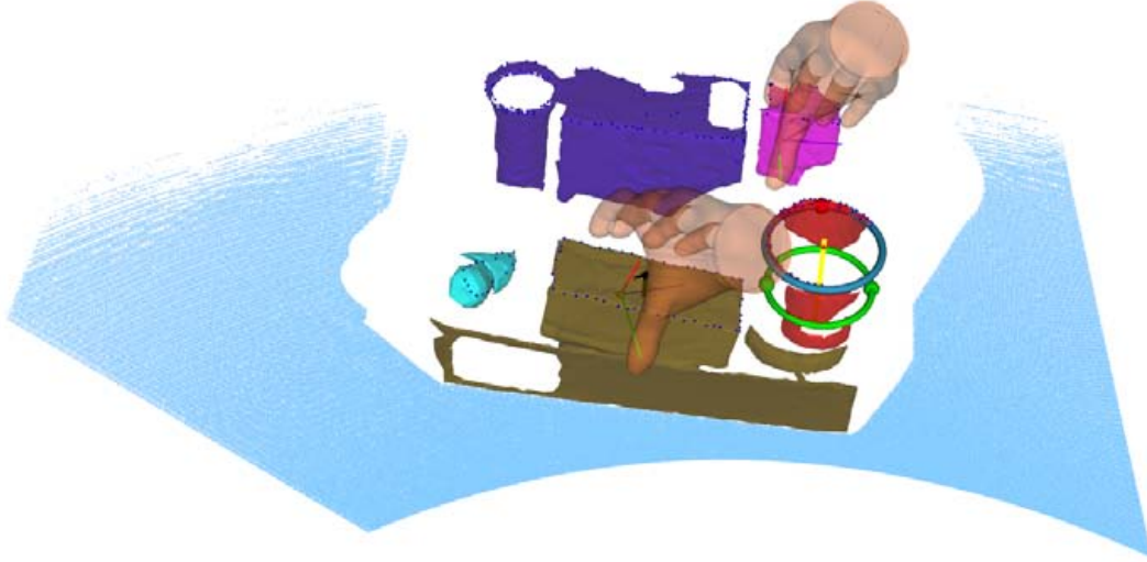
Figure 5.17: Laser data: Detected grasping points and poses of unknown objects in a box. There is a lower detection rate, because of possible collisions of the hand with the box.
