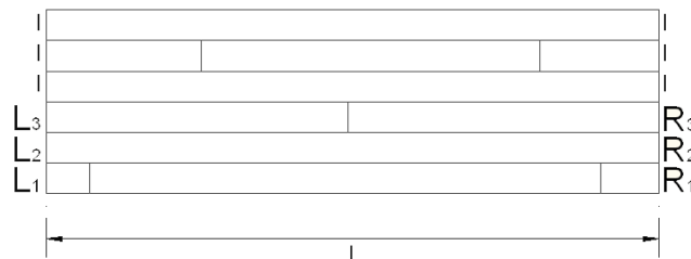
Figure 4.1: Idea of building up a glulam beam with an endless lamella ( l - the length of the glulam beam)
