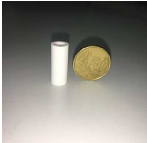
Figure 9: Picture of a 25 mm substrate tube as recieved.
