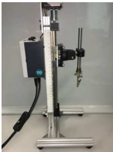
Figure 11: Setup used for dip-coating.
