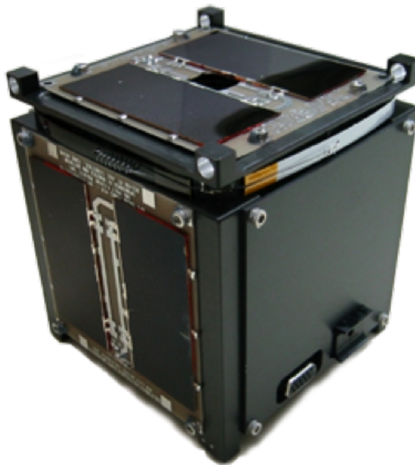
Figure 2.2: The CubeSat CP3 (picture is courtesy of Californian Polytechnical University, San Louis Obispo)
