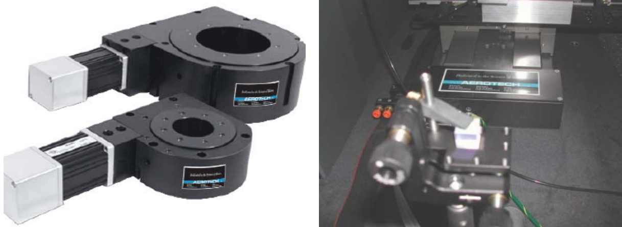
Figure 33: Left picture: Aerotech Rotary Stages type ART 300 (Aerotech, 2009); Right picture: beam splitter
